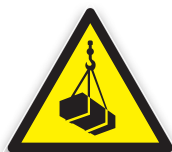
Danger, charges suspendues
